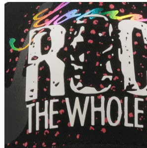
Combination of different techniques of customization: screen print, rubber print, colored foil print
